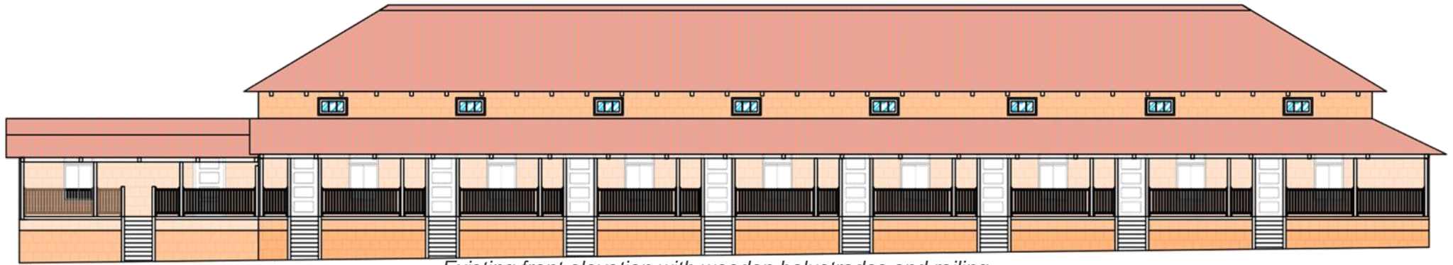
Existing front elevation with wooden balustrades and railing
